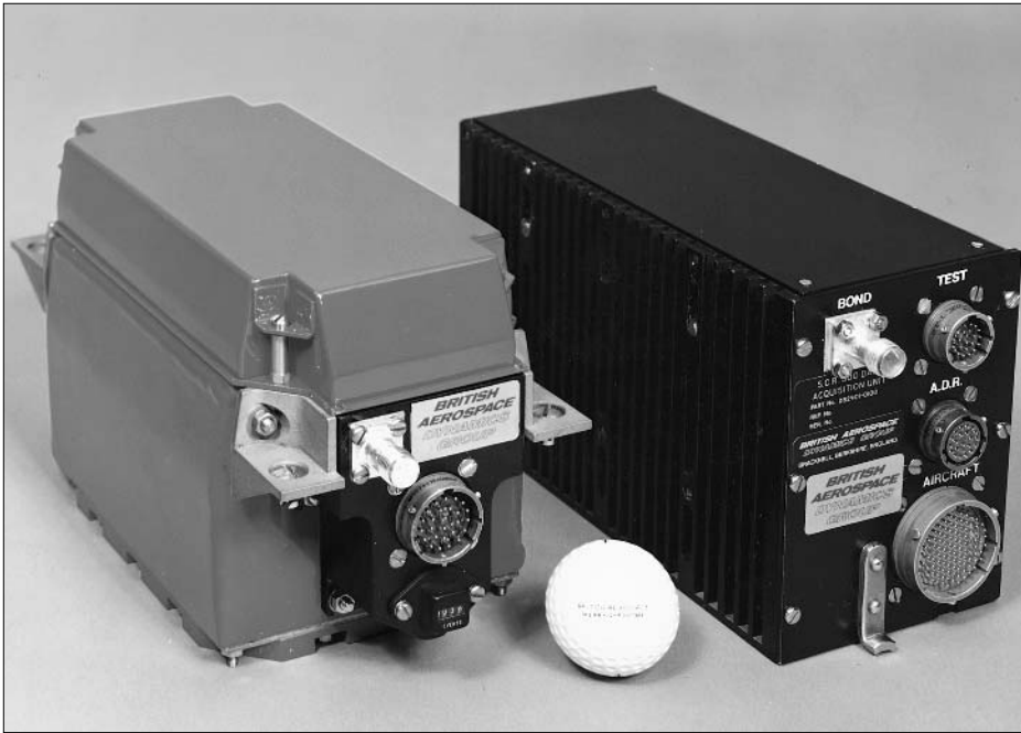
Fig. 8.11 Examples of crash recorders (BAE SYSTEMS)
