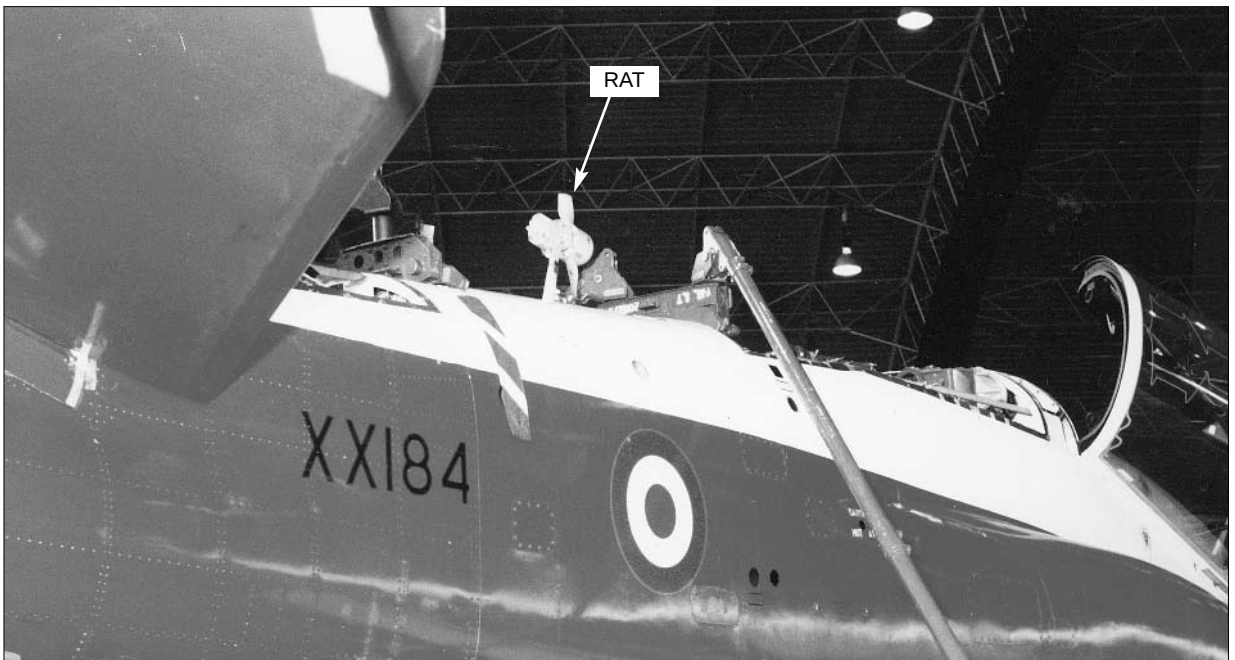
Fig. 4.14 The BAE SYSTEMS Hawk 200 ram air turbine extended (BAE SYSTEMS)
